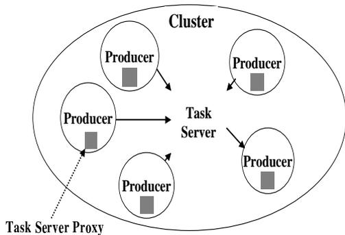
**Figure 3: A Task server and its associated set of Producers.**
